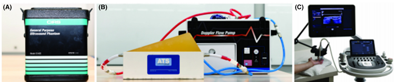
FIGURE 2 Experimental setup and equipment utilized on this study: (A) a general purpose phantom was used for in vitro resolution studies, i.e., the smallest detectable feature (at various depths) available to us through a commercially available phantom; (B) similarly, a cardiac flow pump (left) and Doppler phantom (right) were also utilized in the in vitro study to the slowest detectable flow rate, given the limitations of the flow pump as well as the capabilities of the utilized transducers and imaging modalities; and finally, and (C) the experimental set up for in vivo study, showcasing the participant's hand, the ultrasound probe holder, and a sample scanner
