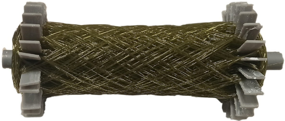
Fig. 10. A tapered mandrel wound with 135 m of fiber and 117 m of length between the two supports. The winding process last 5 h, which can be significantly reduced by increasing the velocity of motors.
