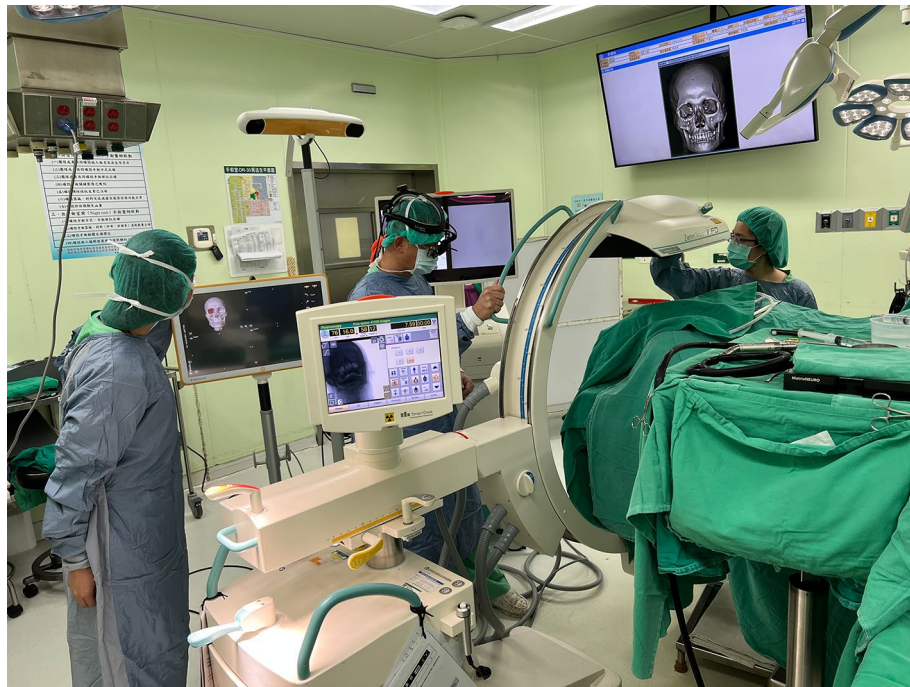
Figure 4. The setup of surgical navigation and intraoperative 3D C-arm computed tomography. The surgical navigation was used as a guide to determine the implant position. After plating, intraoperative 3D C-arm CT was performed to examine the adequacy of zygoma reduction and orbital reconstruction.
