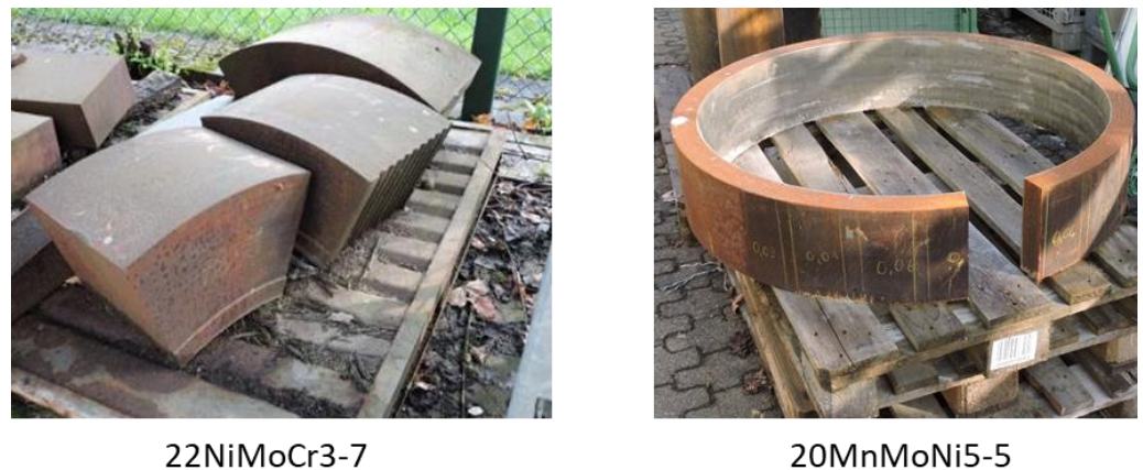
Figure 1. Reactor components provided by Fraunhofer IWM.
