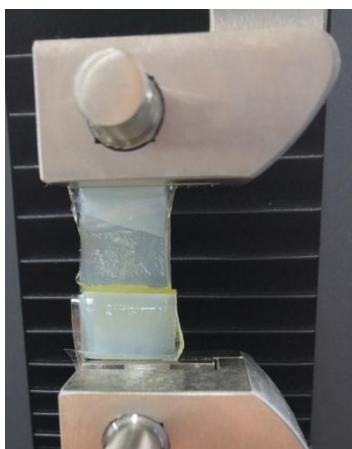
Figure S5 Photo of the peeling test after NIR irradiation. Related to Figure 3 .
