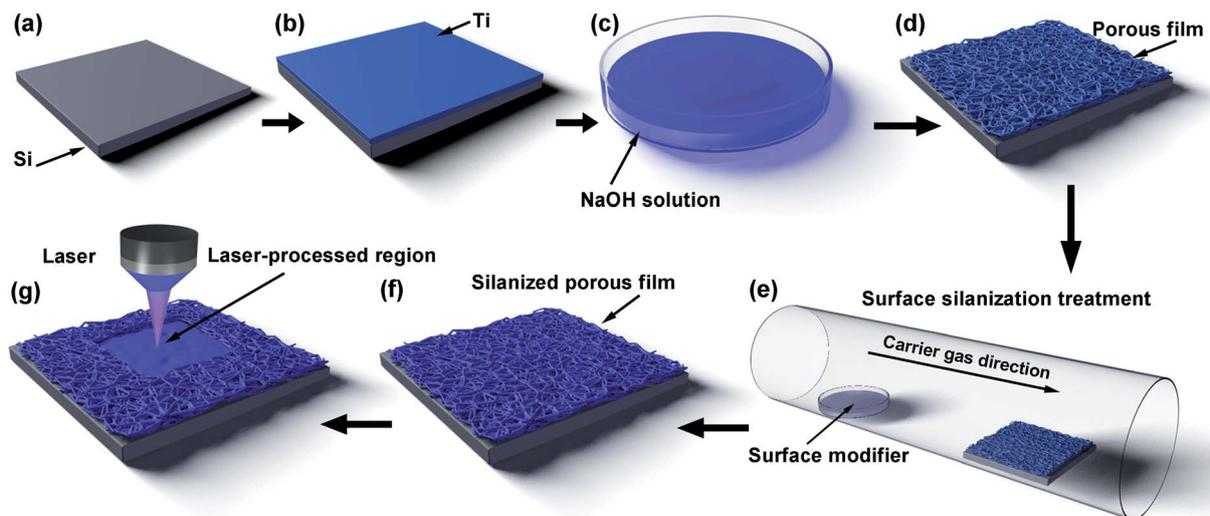
**Fig. 1** Schematic illustration for fabricating surfaces with highly controllable wettability. (a) The Si substrate. (b) The Ti nanofilm deposited on the Si surface. (c) The Ti nanofilm immersed in sodium hydroxide solution for hydrothermal reaction. (d) The porous nanofilm produced on the Si substrate. (e) Surface modification. (f) The silanized porous nanofilm. (g) The laser processing of the porous surface.
