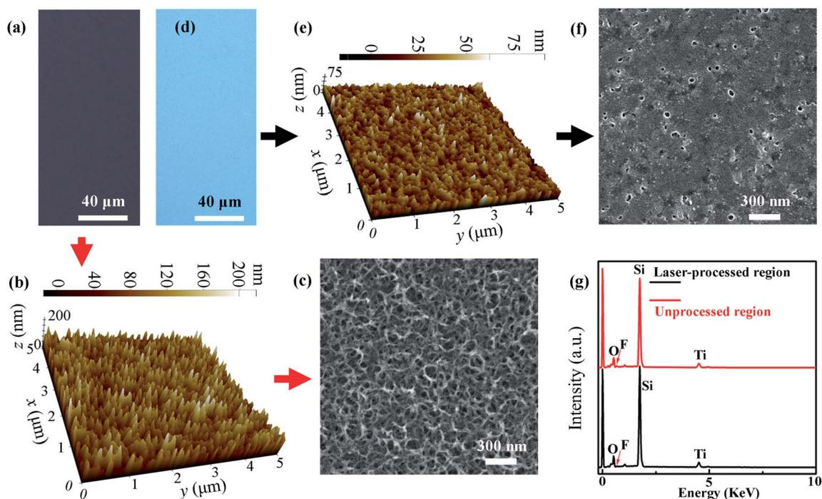
**Fig. 2** (a) Optical image, (b) AFM image and (c) SEM image of a surface in the laser-unprocessed region. (d) Optical image, (e) AFM image and (f) SEM image of a surface in the laser-processed region. (g) EDS spectra of a surface in the laser-unprocessed region (red curve) and of that in the laser-processed region (black curve).
