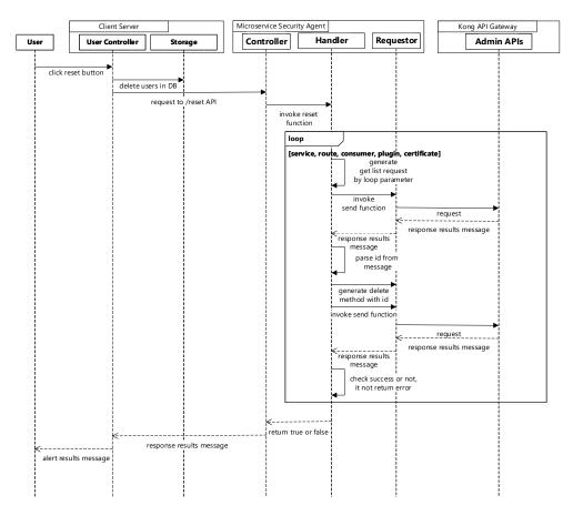
Figure 7. Reset sequence diagram for removing all the configurations.
