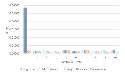
Figure 16. Round trip time for using the microservices API, with and without a token.
