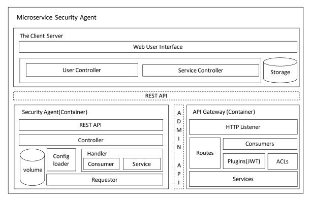
Figure 2. Configuration of the API gateway for microservice security.
