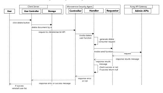
Figure 5. Sequence diagram for user removal.
