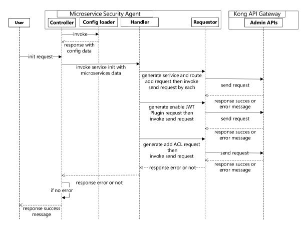
Figure 3. Sequence diagram for microservice security initialization.
