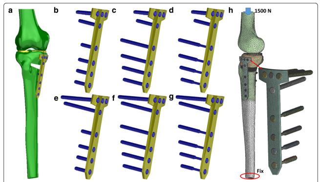
**Fig. 1** a Solid model. Short proximal screw with **b** one-cortical, **c** two-cortical, and **d** far-cortical locking screws. Long proximal screw with **e** one-cortical, **f** two-cortical, and **g** far-cortical locking screws. **h** Boundary condition used in this study
