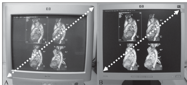
Figure 1 (A,B): Screen sizes. In CRT monitors (A), the screen size is measured diagonally from the outside edges of the display casing. In LCD monitors (B), the screen size is measured diagonally from the inside of the beveled edges. Thus a 17-inch LCD display is comparable to a 19-inch CRT display. The CRT display includes 2 inches of casing, as well
