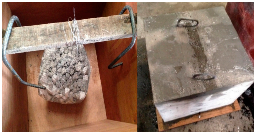
Figure 19. Concrete sample with a honeycomb placed at the center.
