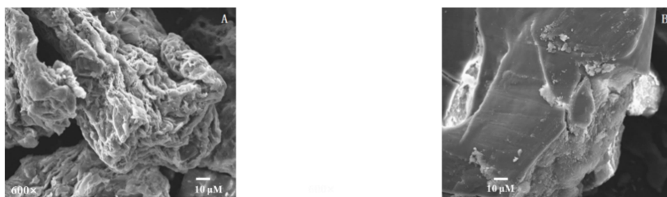
Figure 2. Scanning electron microscopy (SEM) images of SP (A: treated by steam explosion at 2.0 MPa, 88 s and 60 mesh untreated, B: original).
