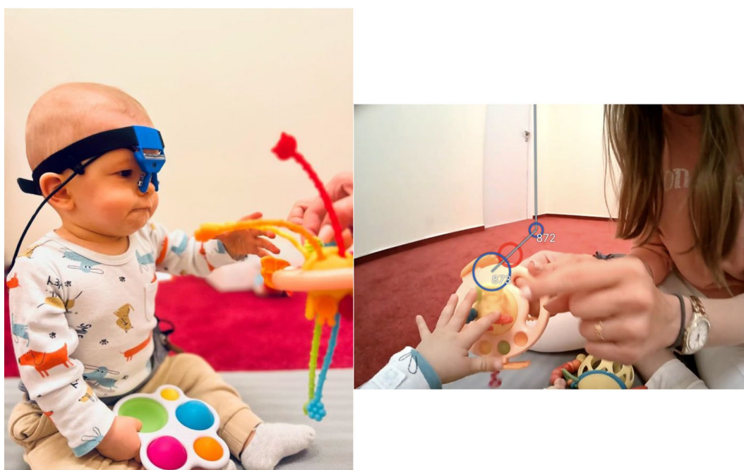
Fig. 1 Positioning of the wearable eye-tracker on an infant's head (left) and an example frame from the eye-tracking recording (right). The images are displayed with permission from the caregiver
