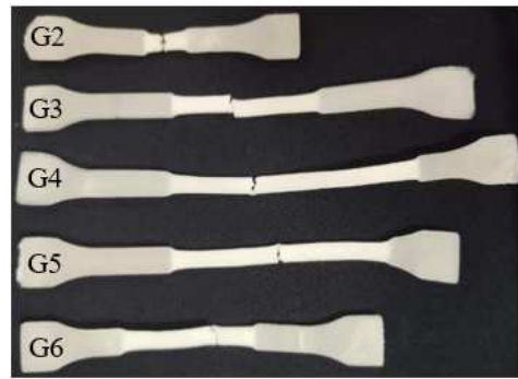
Figure 12. Tensile splines of the PLA/PPC/PLA-g-GMA blends (G2: PLA/PPC; G3: PLA/PPC/PLA-g-GMA; G4: PLA/PPC/PLA-g-GMA/St; G5: PLA/PPC/PLA-g-GMA/AMS; G6: PLA/PPC/PLA-g-GMA/EP).
