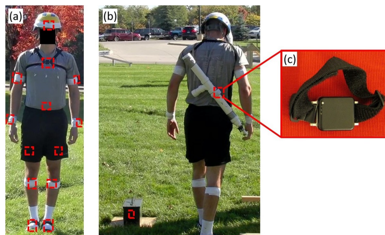
Fig 1. Participant outfitted with equipment (unloaded condition). (a) Participant wearing an array of IMUs (red rectangles) attached to major body segments and in the approximate locations shown (sacrum IMU on posterior). (b) Participant with the mock rifle slung over the shoulder with additional IMU nodes attached to the mock rifle and embedded in the ammo can. (c) Image of single IMU node with integrated Velcro strap.
