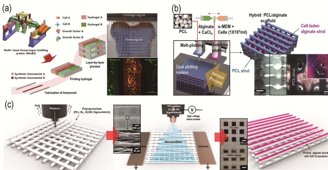
**Figure 5.** Hybrid modifications of the 3D cell printing process with (a, b) a multi-nozzle system using natural and synthetic polymers ((a) Shim *et al.*<sup>[53]</sup>, (b) Lee *et al.*<sup>[54]</sup>) and (c) an additional electrospinning process for surface alignment (Yeo *et al.*<sup>[56]</sup>).
