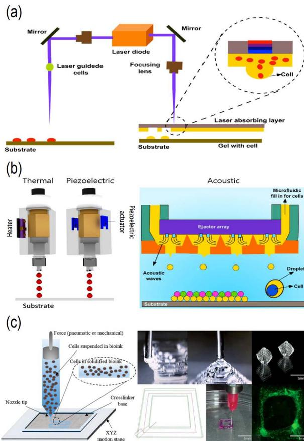
**Figure 1.** Basic techniques of 3D cell printing, (a) laser-assisted 3D cell printing techniques with and without an absorbing layer,<sup>[17,22]</sup> (b) thermal, piezoelectric, and acoustic inkjet 3D cell printing systems,<sup>[22,28]</sup> and (c) microextrusion 3D cell printing systems and products<sup>[14,35]</sup>.
