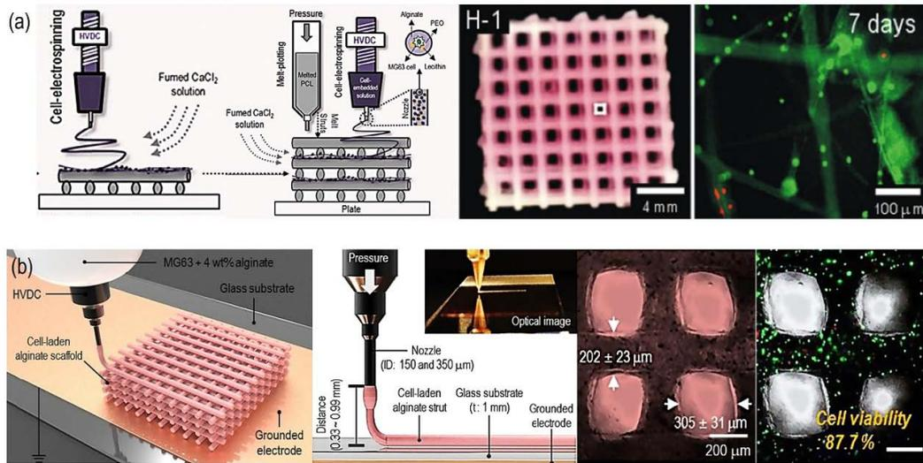
**Figure 4.** (a) Electrically operated cell printing modification supplemented with the aerosol crosslinking process<sup>[51]</sup> and (b) extrusion-based cell printing with an electric field (1 to 3 kV in 0.33 to 0.99 mm)<sup>[52]</sup>.
