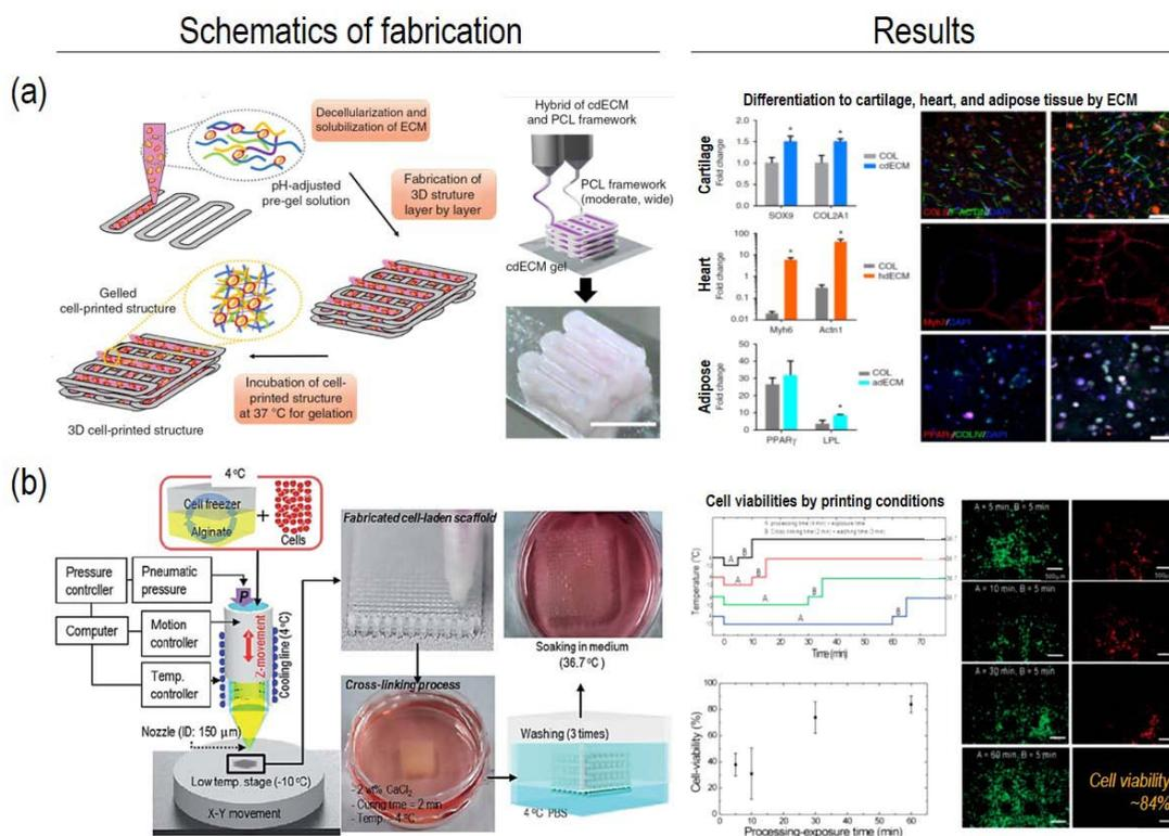
**Figure 3.** Temperature-controlled 3D cell printing process, (a) increasing temperature-controlled (from 4 to 37°C) printing using ECM-based bioinks [48, 49] and (b) low-temperature (−10°C) cell printing process [50].
