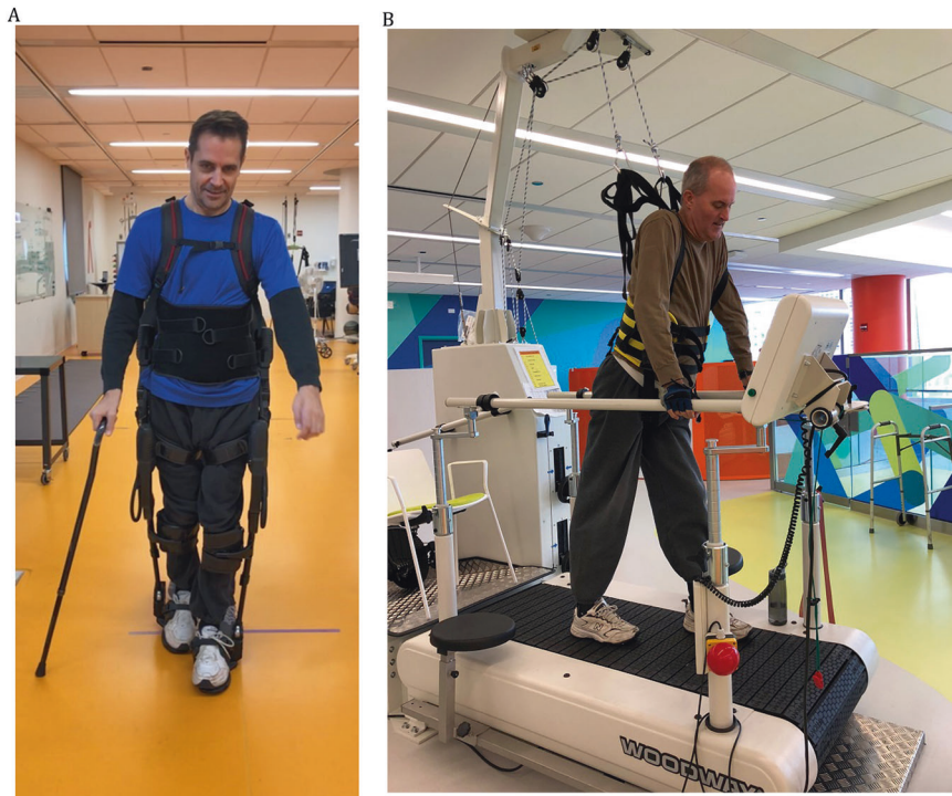
Fig. 1 Electromechanical devices used for the active intervention groups. A Photograph with permission, showing an SCI participant training in the robotic exoskeleton suit. B Photograph with permission, showing an SCI participant from the Active Control group training using the body weight supported treadmill prior to overground stepping practice.
