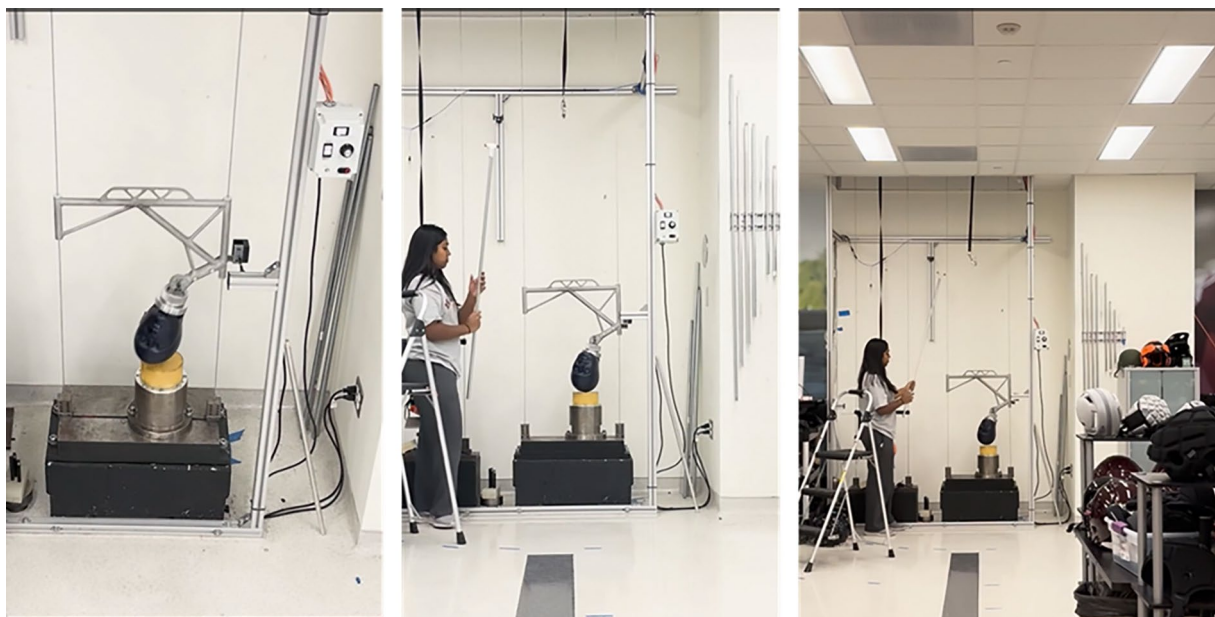
Fig. 1 Guided NOCSAE drop tower taken from different camera positions where observed speeds were captured with a speed gate and recorded. The left image was taken from a 2.8 m height, 3 m distance, and 55-degree camera angle. The middle image was taken from a
