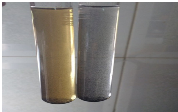
Fig. 1 Brown coloured solution (plant extract) changes to black (reduced graphene oxide nanoparticles) confirms the formation of graphene nanoparticle
