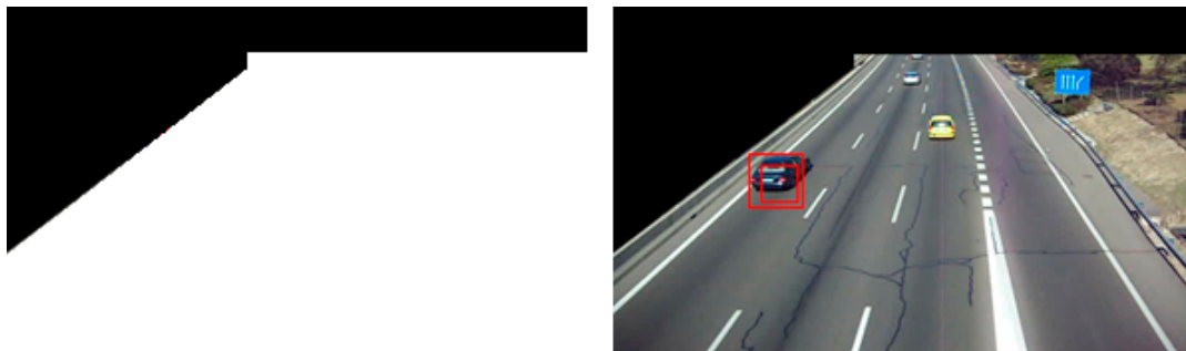
Figure 2. GRAM dataset: (left) a pixel mask that highlights the Region of Interest about vehicles present, annotated (and subsequently trackable) in each video frame (right).
