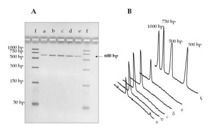
**Figure 6.** (A) Agarose gel electrophoresis images of 600 bp PCR products generated from purified *E.coli* gDNA using the PPC microchip, and (B) 2D traces of the electropherograms in the accompanying image. Samples were immobilized to the capture bed in 3% PEG, 0.4 M NaCl and 70% ethanol. Lanes a–e, chip#1–5 and lane (f) DNA sizing ladder. The sample volume loaded onto the gel was 5  $\mu$ l with 1  $\mu$ l of the loading dye. Separation parameters are described in Figure 4.
