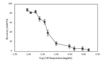
**Figure 5.** The recovery of gDNA loaded onto the microchip using the PPC-SPRI purification assay for *E.coli* gDNA, which was immobilized to the activated surface using 3% PEG, 0.4 M NaCl and 70% ethanol. The total DNA mass before and after PPC-SPRI was estimated from absorbance values at 260 nm and fluorescence data. Error bars in the graph represent SDs from three replicate runs.
