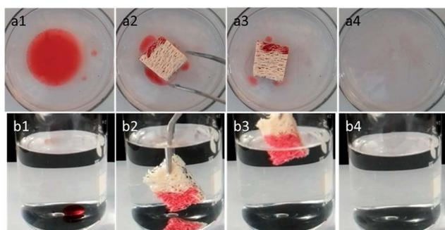
Fig. 5 Optical photos demonstrating the processes for oil–water separation of the as-prepared loofah: (a) sequential snapshots of removing a layer of oily red dyed *n*-hexane on top of water and (b) sequential snapshots of removing oily red dyed chloroform under water.
