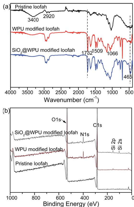
**Fig. 1** FT-IR spectra (a) and XPS spectra (b) of pristine loofah, WPU modified loofah, and SiO<sub>2</sub>@WPU modified loofah.
