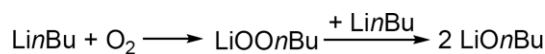
Scheme 13. Reaction of n -butyllithium with molecular oxygen. The initially formed lithium n -butyl peroxide reacts with excess alkyllithium to lithium n -butanolate.
