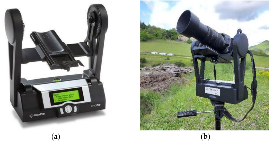
Figure 2. GigaPan acquisition system used at PBL: (a) GigaPan robotic head with screen and controls; (b) GigaPan system equipped with a Nikon D5000 camera and 300mm telephoto lens.
