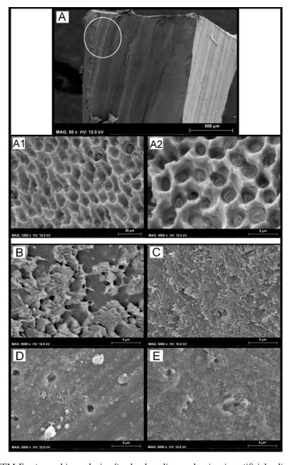
**Figure 3.** SEM Fractographic analysis after load cycling and aging in artificial saliva. **(A)** SEM fractography of a specimen created with SCU applied in ER mode and restored with RC showing
