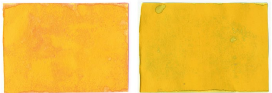
Fig. 12 UIP confirmation of citric acid presence (red) on top surface of first filter (left) and underside of first filter (right) showing no citric acid. Due to the need for rehydration in this assessment, the right image shows the alkaline nature of water
