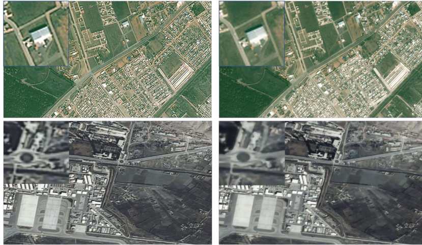
Figure 4. Output of the super-resolution convolutional neural network (SRCNN) using a different training set with “Jilin-1” satellite video ( left ) and Yang91 ( right ). Yang91 is a standard training set that was firstly used by Yang [3].
