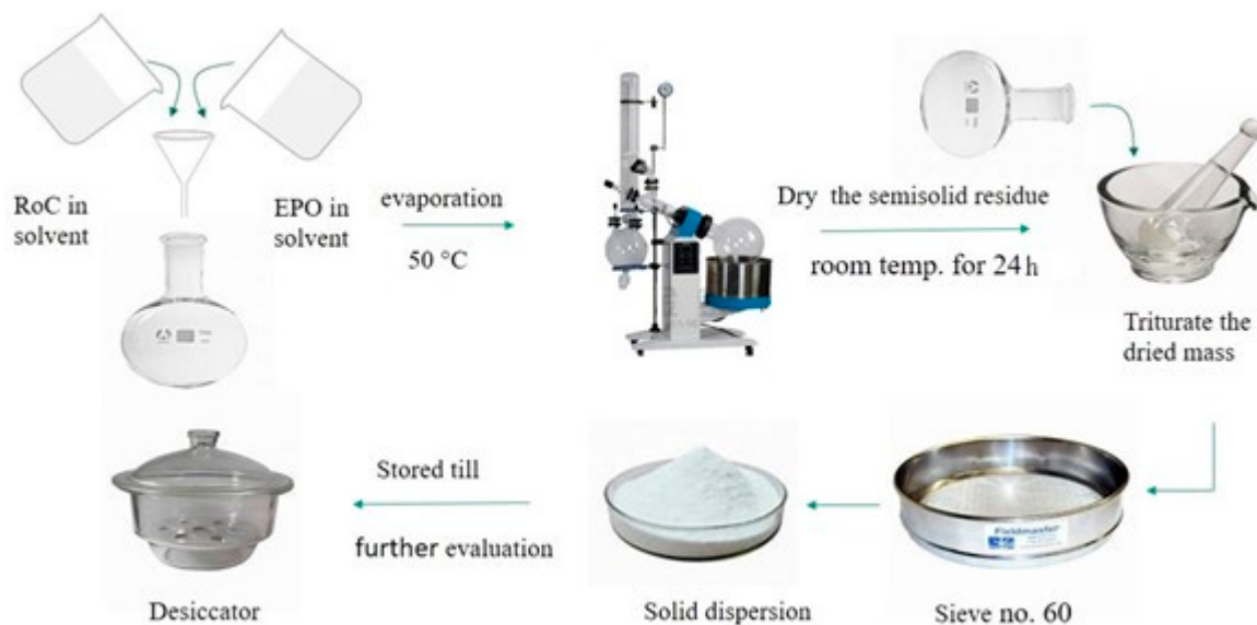
Figure 17. Diagrammatic presentation for the manufacturing process of solid dispersion of RoC using SE technique.
