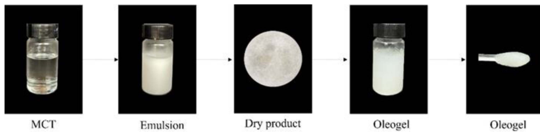
Figure 4. The process of preparation for oleogels.
