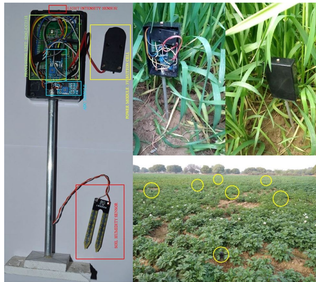
Figure 1. Sensor node prototype and deployment in T^{wheat} and T^{potato} .
