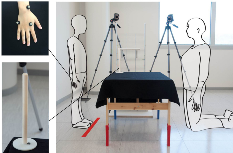
Fig. 1. A schematic representation of materials and experimental set-up that were used to test grasp height effect. The position of the markers on the participant's right hand and the cylinder were used to measure the grasp height effect during the unimanual, bimanual, and joint tasks.
