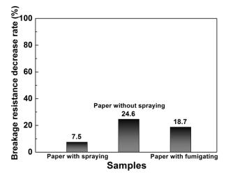
**Figure 8.** The impact of paper breaking resistance with and without the photocatalytic bactericidal spray, with potassium permanganate and formaldehyde fumigation.
