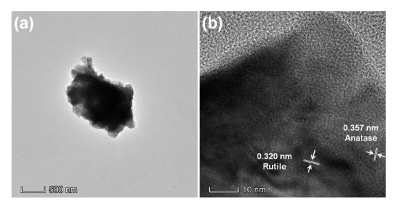
Figure 4. (a) TEM and (b) HRTEM images of TiO<sub>2</sub>-750.
