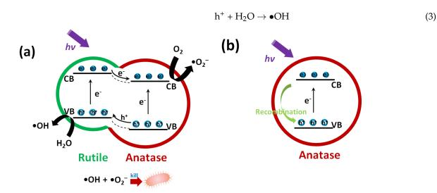
**Figure 7.** The photocatalytic antibacterial mechanism of  $TiO_2$  nanospheres (**a**) with and (**b**) without rutile/anatase heterojunctions. Adapted with permission from ref. [10]. 2020 Elsevier.
