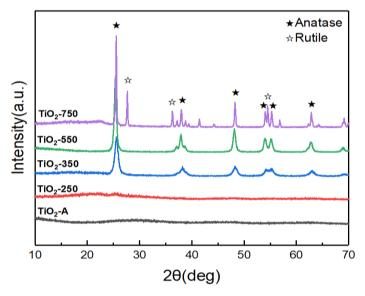
**Figure 1.** XRD patterns of TiO<sub>2</sub>-A, TiO<sub>2</sub>-250, TiO<sub>2</sub>-350, TiO<sub>2</sub>-550, and TiO<sub>2</sub>-750.
