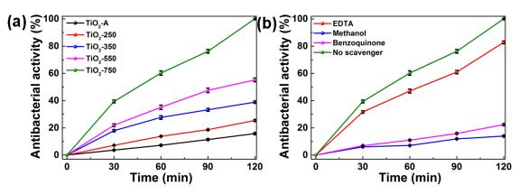
**Figure 6.** (a) Photocatalytic antibacterial efficiency against *E. coli* for  $TiO_2$ -A,  $TiO_2$ -250,  $TiO_2$ -350,  $TiO_2$ -550, and  $TiO_2$ -750 under simulated solar light irradiation; (b) reactive species trapping experiments of  $TiO_2$ -750 under simulated solar light irradiation. Error bars represent the standard deviation of three independent experiments.
