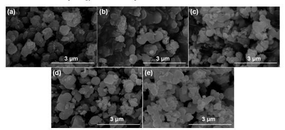
Figure 3. SEM images of (a) TiO<sub>2</sub>-A, (b) TiO<sub>2</sub>-250, (c) TiO<sub>2</sub>-350, (d) TiO<sub>2</sub>-550, and (e) TiO<sub>2</sub>-750.
