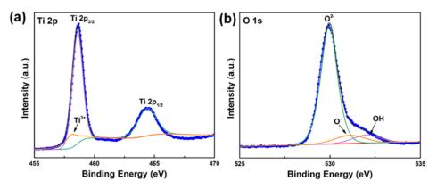
Figure 2. (a) Ti 2p and (b) O 1s XPS spectra of TiO<sub>2</sub>-750.
