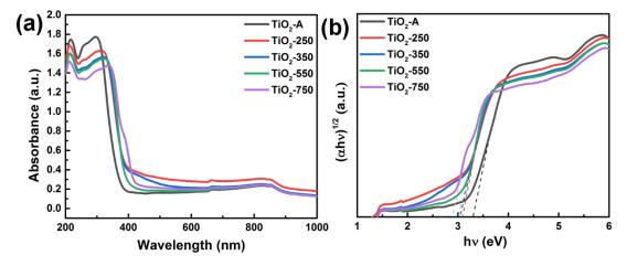
Figure 5. (a) UV-Vis absorption spectra and (b) bandgap value of TiO<sub>2</sub>-A, TiO<sub>2</sub>-250, TiO<sub>2</sub>-350, TiO<sub>2</sub>-550, and TiO<sub>2</sub>-750.
