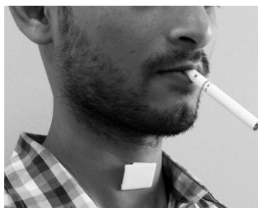
Figure 7. Acoustic sensor attached to the suprasternal notch to detect smoke related breathing.
