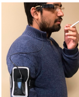
Figure 8. Egocentric camera attached to the eye-glass temple to captured details of smoking event.
