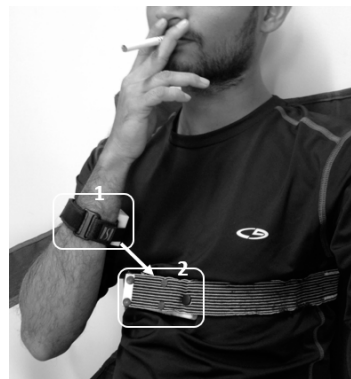
Figure 4. The concept of proximity sensor: Closeness of hand to mouth, i.e., the closeness of module 1 to module 2.
