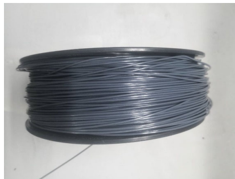
Figure 3. FDM 3D printed special PEEK/tungsten shielding materials.
