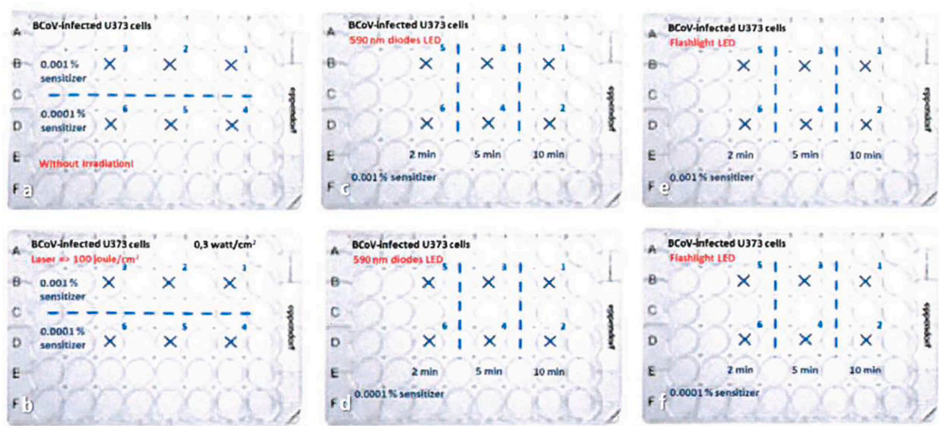
Fig. 2. Schematic representation of the individual approaches per plate for the treatment of the BCoV-infected cells Treatment of the cells with sensitizer only (a), photodynamic treatment with laser (b), 589 nm LEDs (c, d) and flashlight (e, f).
