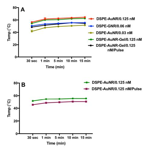
**Figure 8.** Temperature induced by NIR laser excitation of DSPE-AuNR suspensions over 15 min. (**A**) Temperature of DSPE-AuNR suspension at three different molar concentrations, DSPE-AuNR loaded into hydrogel upon excitation with CW or pulse laser (3 W cm<sup>-2</sup>). (**B**) Temperature of DSPE-AuNR suspension upon excitation with 1 W cm<sup>-2</sup> of CW or pulse laser. The initial temperature was 19.6 ± 1.1 °C. Data are presented as mean ± SD (*n* = 3).
