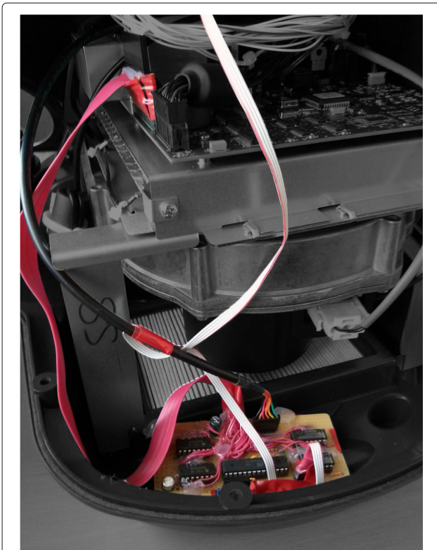
Fig. 2 Add-on board integration to 3M Bair Hugger. Image of the opened 3M Bair Hugger device with the installed add-on board for reading the current device state and remote control of the switches. Original 3M Bair Hugger parts, desaturated in color image
