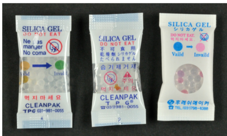
Figure 3 Examples of three silica gel sachets. Left: partial-indicating silica gel, with instructions for interpretation. Center: partial-indicating silica gel, no instructions for interpretation. Both sachets (left and center) are packed in a transparent but vapor-impermeable plastic preventing uptake of humidity. Right: vapor-permeable sachet with inspection window. Note warning message written in multiple languages – mandatory in CE-marked products - (sachet at the left) and the pictogram “Do not eat” (all three sachets) which is not clear on the sachet at the right.
