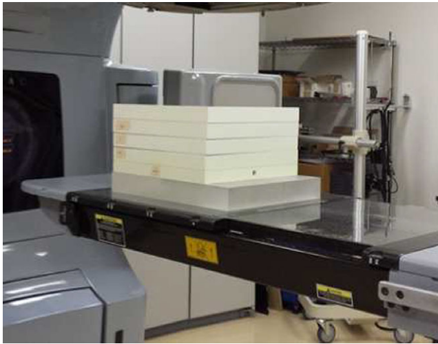
Fig. 2. Example of the phantom geometry used to measure TPRs . Normally, the manufacturer provides one slab for buildup, one slab for chamber insert, and one slab for backscatter in order to measure the absorbed dose at a depth of 4.25 cm in PMMA and 4.95 cm in PWDT for the cross-calibration of Delta4. This figure shows four PWDT buildup slabs, one PWDT chamber insert slab (SCD = 100 cm, depth = 15.45 cm), and one PMMA slab for backscatter. The manufacturer provides only PMMA for the backscatter slab. In this study, several sets of the calibration slab phantoms were stacked to measure TPRs at several depths. To calculate TPRs in the Monte Carlo simulation and RTPS, the geometry and phantoms were modeled the same as the geometry of the measurements.
