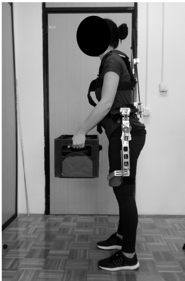
Figure 1. SPEXOR passive spinal exoskeleton, as used during a lifting task.
