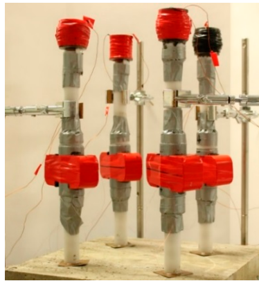
Figure 10. Concrete test setup. Photo of the four transducers placed above one of the eight samples.
