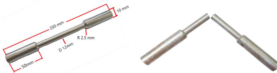
Fig. 1. a) Prepared tensile test sample and b) Sample after tensile test performed.
