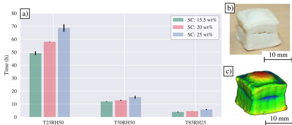
Figure 2. (a) Bar graph showing the drying times of the tested samples, (b) Photograph of cracked sample (20 wt% EFCNF dried at 85 °C and 25% relative humidity), (c) Visualization of drying deformation of sample shown in Fig. 2b, where red, green and blue colors denote positive, low and negative error from a fitted box-like shape respectively.
