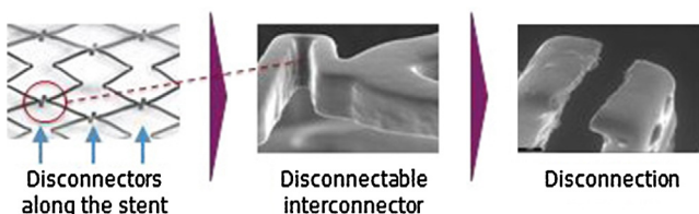
Fig. 4 – Design aspects of Stentys™ stent.
