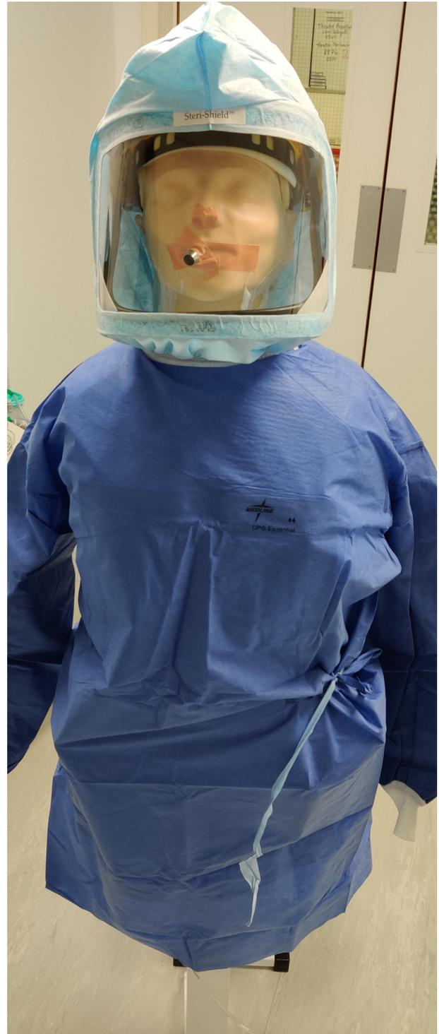
**Figure 1.** Experimental set-up using a mannequin with a particulate detector sealed at the mouth of the mannequin.
