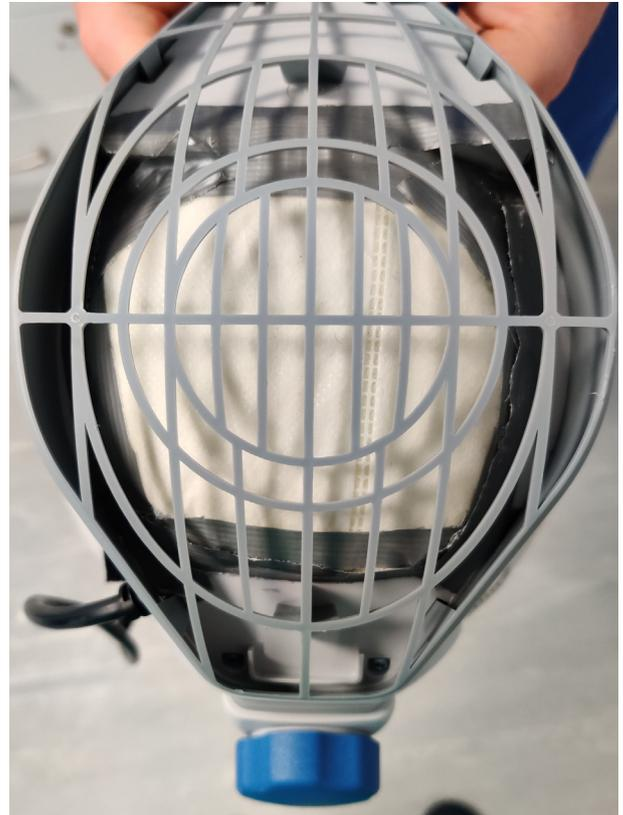
Figure 3. Stryker Flyte T5 helmet with high-efficiency particulate air filter cut to size for fan inlet with plastic grill intact.
