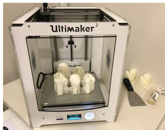
Fig. 1 3D printing models of proximal humerus fractures using CT scans as a model
