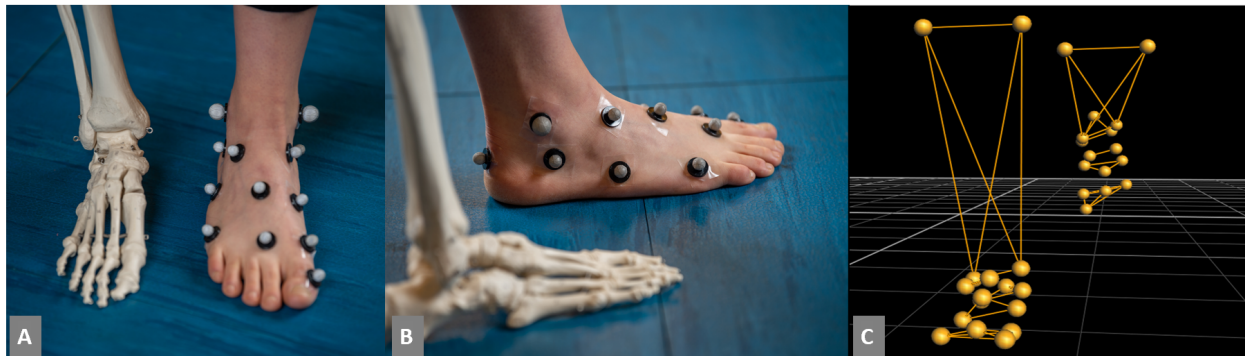
Figure 1. (A) and (B) Photograph of reflective marker locations on a participant's feet, and (C) Single frame image of reconstructed three-dimensional marker trajectories from the Vicon motion capture system.
