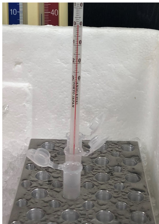
Fig. 1. An aluminum rack kept on ice. To ensure temperatures at 1°C or at -20°C, all reactions were performed in aluminum racks. For the 1°C experiments, the racks were placed on ice; for the -20°C experiments, the racks were kept in a -20°C freezer and removed from the freezer to a safety cabinet on ice. After solutions were added, the racks were immediately returned to the freezer.
