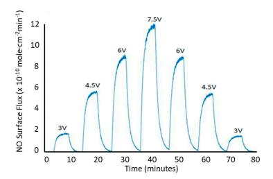
**Figure 2.** Nitric oxide (NO) release profile of SNAP-HPAMAM blended in polyvinyl chloride (PVC) using photoinitiation using a 470 nm LED and a 130  $\Omega$  resistor and different applied voltages as noted on the face of the graph.
