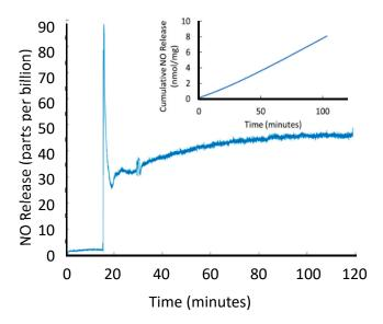
**Figure 4.** Passive NO release of SNAP-HPAMAM (2 mg per film) encapsulated in PVC in 2 mL of PBS at 37 °C.
