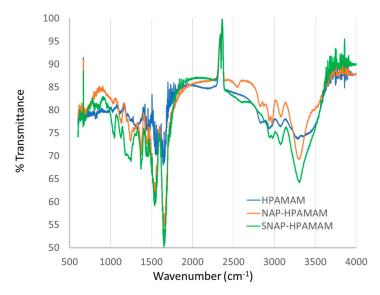
**Figure 5.** FTIR analysis of HPAMAM (blue), NAP-HPAMAM (orange), and SNAP-HPAMAM (green) compounds, the double spike that appears near 2400 cm<sup>-1</sup> is an instrument artifact and used to align spectra.
