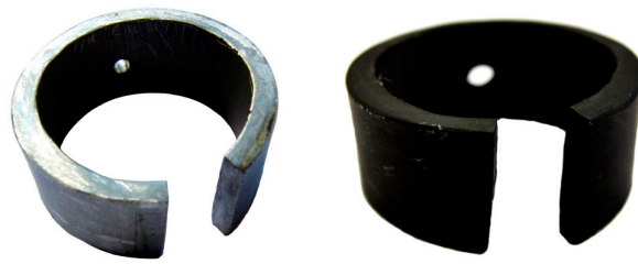
Figure 9. Depiction of the Inconel 600 alloy ring: before (left) and after the oxidation-lithiation process (right).
