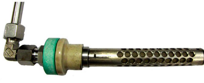
Figure 7. View of the Model III anode construction before the lithiation process.
