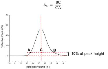
**Figure 5.** The asymmetry factor (As) measures the peak tailing and is defined as the distance from the center line of the peak to the back slope divided by the distance from the center line of the peak to the front slope, measured at 10% of the maximum peak height.
