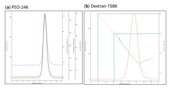
**Figure 8.** MWD plot measured by high-performance size exclusion chromatography (HPSEC) (OMNISEC) of standards: (a) PEO-24K for light scattering/triple detection calibration, (b) Dextran-T68K for validation of the calibration, with excellent agreement  $M_w$  vs. retention time (mL) relation ( $M_w$  (Dextran-T68K)<sub>Malvern</sub> = 68162 ± 450 Da,  $M_w$  (Dextran-T68K)<sub>Validation</sub> = 66807 ± 291 Da).
